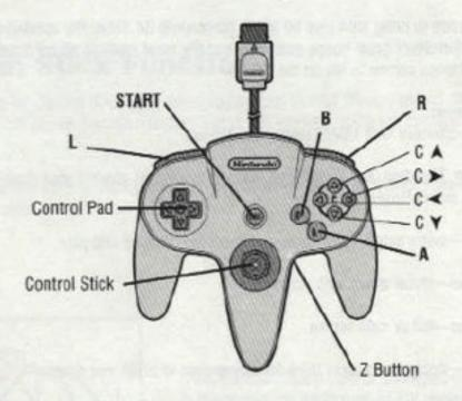
Note: The Control Stick functions identically to the Control Pad throughout all menus and gameplay. Also: during gameplay the Z and L buttons activate the same actions. In this manual, when L is mentioned, you can also use the Z Button.
