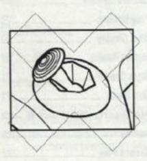
If the Control Stick is held at an angled position (as shown in the picture on the left) when the power is turned ON, this position will be set as neutral. This will cause games using the Control Stick to operate incorrectly.
